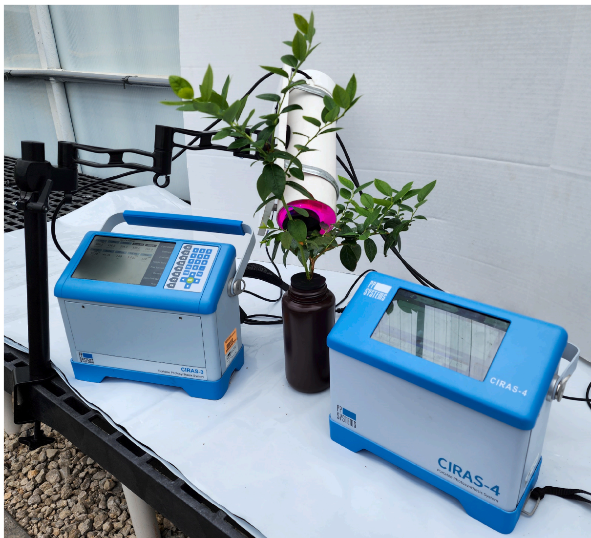
Fig. 1. Gas analysis system used to simultaneously measure blueberry branch net photosynthesis ( A_{\text{branch}} ) and root respiration ( R_{\text{root}} ).
